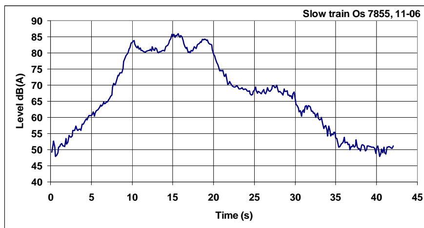
Figure A2-5 Measured LAF levels – L_{eq} = 77,1 dB(A) with T = 42 s
