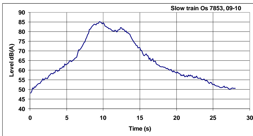
Figure A2-6 Measured LAF levels – L_{eq} = 75,8 dB(A) with T = 28 s
