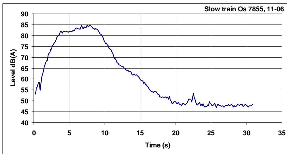
Figure A2-4 Measured LAF levels – Leq = 76,3 dB(A) with T = 30,9 s
