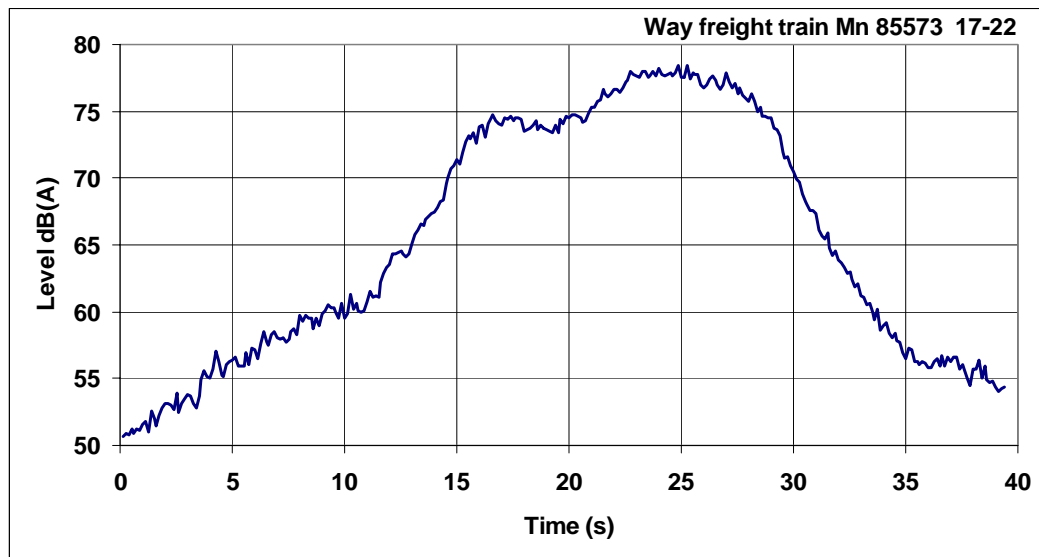
Figure 34: Measured LAF levels – L_{eq} = 71,9 \text{ dB(A)} with T = 39,4 \text{ s} 1462 trains/16h – 19005 carriages/16h
