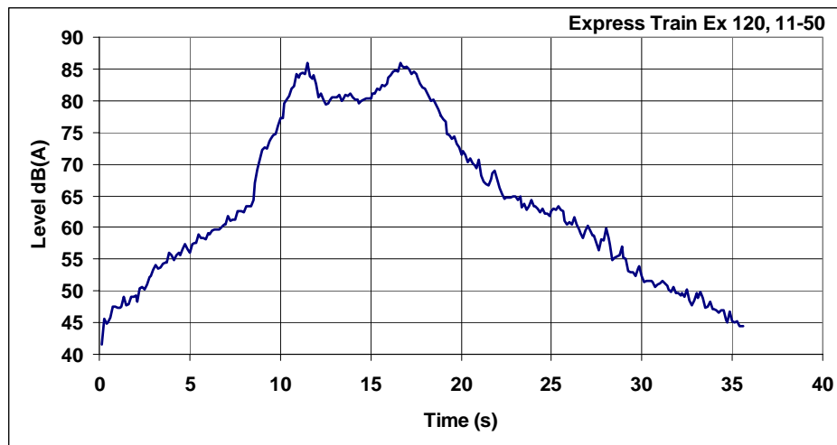
Figure 7: Measured LAF levels – Leq = 76,6 \text{ dB(A)} with T = 35,6 \text{ s} (1618 trains/16h)
