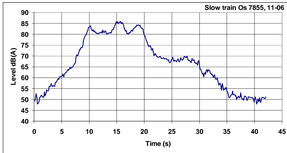
Figure 9: Measured LAF levels – Leq = 77,1 \text{ dB(A)} with T = 42 \text{ s}
