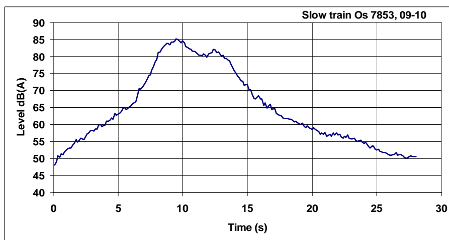
Figure 10: Measured LAF levels – Leq = 75,8 \text{ dB(A)} with T = 28 \text{ s}
