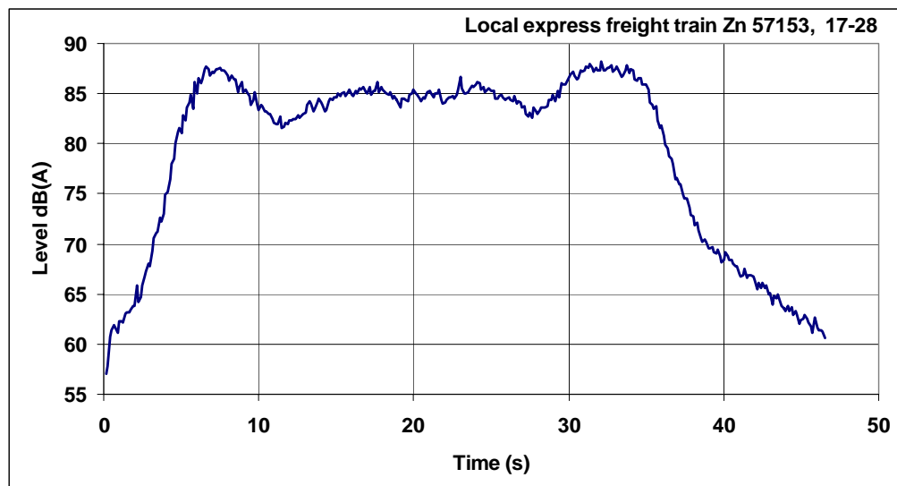
Figure 26: Measured LAF levels – L_{eq} = 83,6 dB(A) with T = 46,5 s 1239 trains/16h – 53264 carriages/16h
