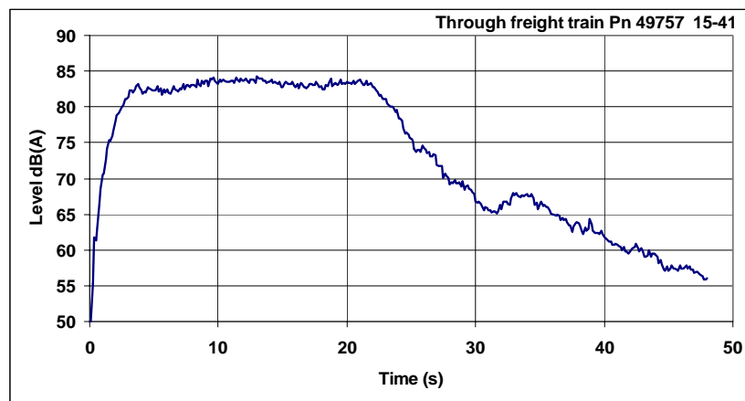
Figure 31: Measured LAF levels – Leq = 79,7 dB(A) with T = 48,0 s 1200 trains/16h – 38400 carriages/16h
